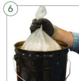
6 SEAL DRUM LINER Gather the liner at the top of the drum, twist and secure with the zip tie.
