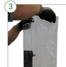
3 PROTECT BATTERIES Place each affected battery/device into a bag and seal. 1 battery/device per bag.
