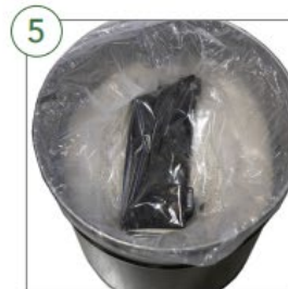
PACK DRUM Place the any remaining CellBlock into the drum. Do not over fill. Any remaining can be used later.
