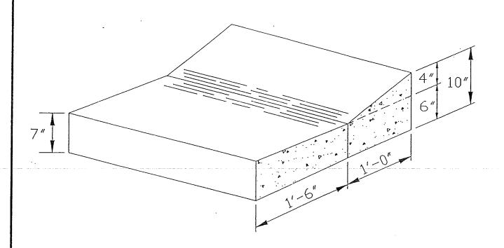
CONCRETE MOUNTABLE CURB & GUTTER DETAIL
